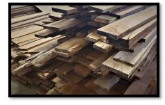
**Poor Quality:** Hobby milled and thickness variations > .25", air dried, poorly stack, warped, water damage and splintering
