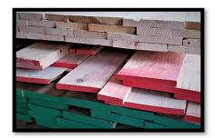
**Graded/Sorted Lumber:** Professionally milled flat with thickness variation < .125", kiln dried, sorted and graded for desired quality.
